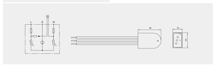
■ Type 3 surge arrester is installed between LPZ2 and LPZ3, it can provide protection for equipments.
